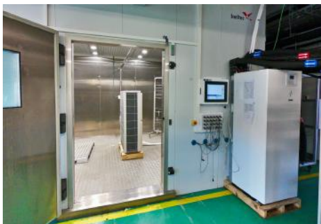
Heat pump in our testing lab
